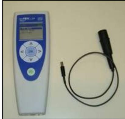
The function checker consists of a combined discharge and ultrasonic source which is energised via the charger socket on the UltraTEV Plus+.
