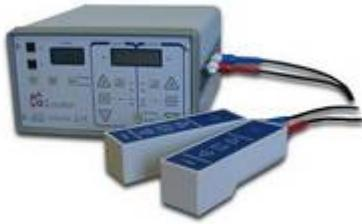
The PD Locator can be used in single probe mode for TEV magnitude measurements, or double probe mode to accurately locate the source of PD activity using the time of flight technique. The PD Locator can measure PD magnitude over a large range with high accuracy and is the benchmark instrument for the assessment of partial discharge activity.
