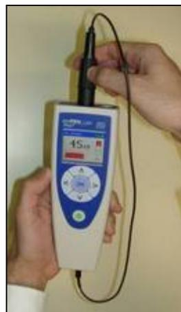
Disconnect the function checker after checking the UltraTEV Plus+; do not attempt to use the UltraTEV Plus+ with the checker plugged in.
